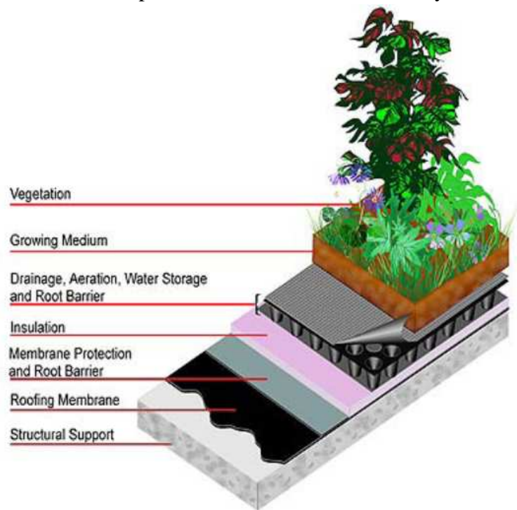
Figure 1: Structure of a Green Roof (Source: heatusa.com)
