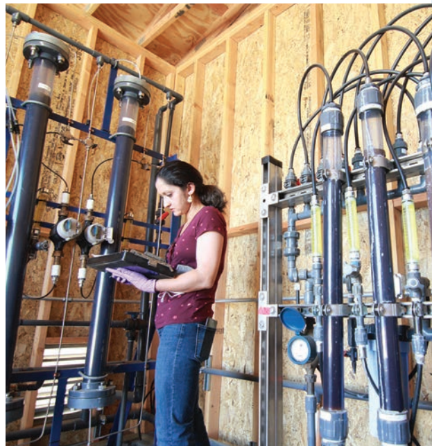
Orange County Water District addressed PFAS in the groundwater basin, including launching the nation’s largest pilot project to test 14 different types of treatment media and identify reliable and cost-effective treatment technologies.
