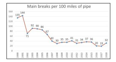
The majority of the main breaks occur in older cast iron pipe. While the utility has not used the material since the 1970s, it still comprises a substantial part of the pipe material in the system.
