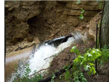
Failure of the 60-Inch PCCP Transmission Main between BE Payne Plant and English Station Road Tank 05/13/09
