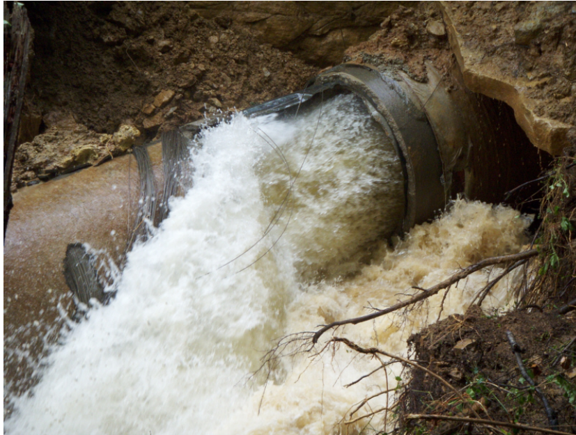
Failure of the 60-Inch PCCP Transmission Main between BE Payne Plant and English Station Road Tank 05/13/09
